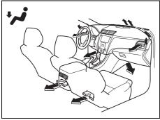
Temperature-controlled air comes out of the floor, rear floor and the side outlets, also comes out of the windshield defroster outlets and also comes slightly out of the side defroster outlets and the side outlets.
